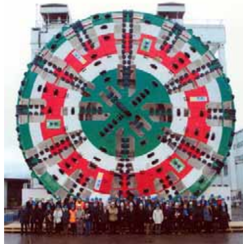
Fig. 1 EPB TBM “Martina”, Diam. = 15.62 m
