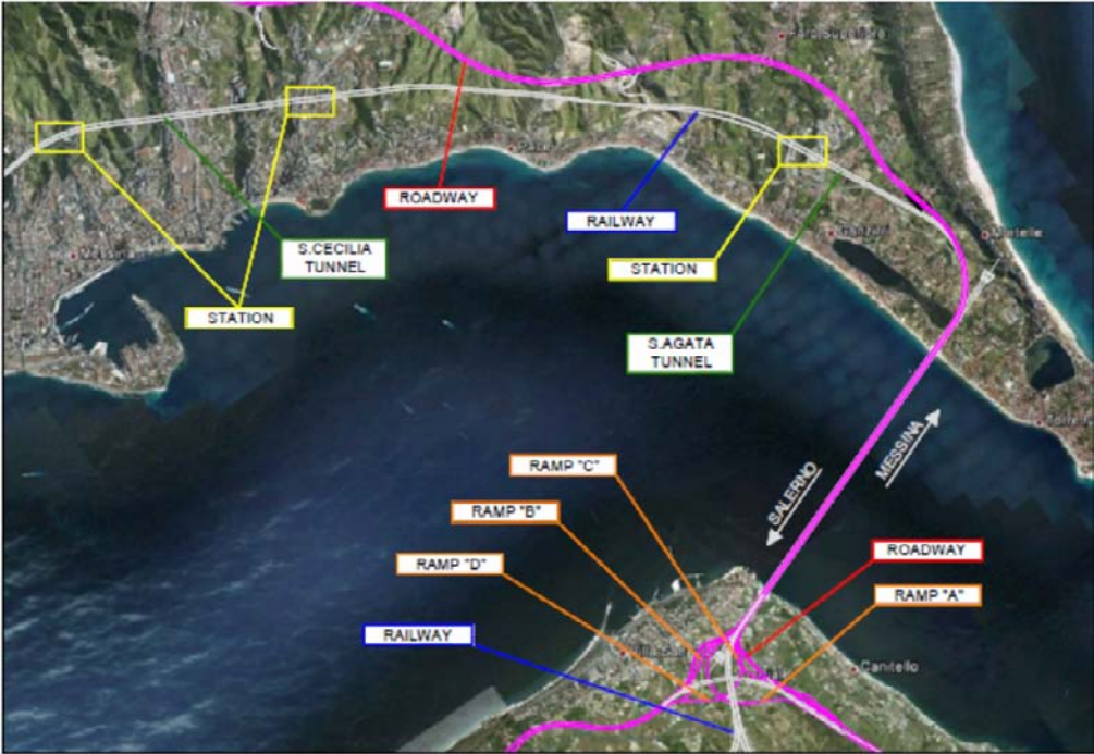
Figure 1. The Main Works
