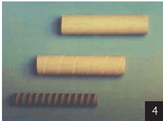
4. SAMPLES OF SMOOTH AND CORRUGATED FIBRE GLASS TUBES
